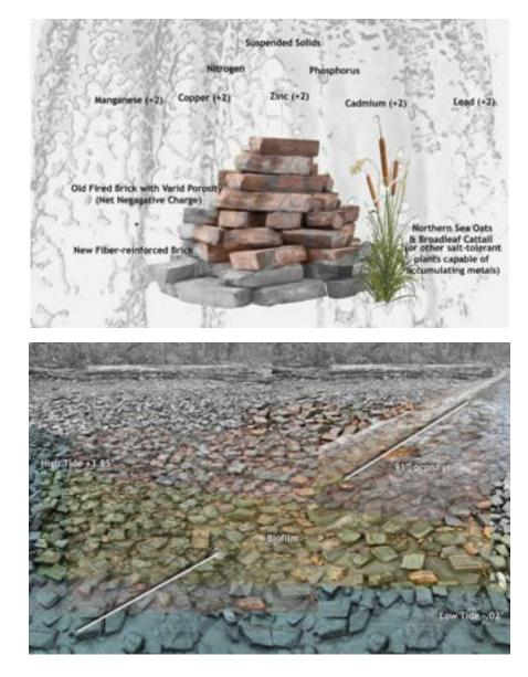
Top: Filtration Capacity of Brick Positively charged heavy metals in this area include cadmium, copper, arsenic, cobalt, and zinc. Bottom: Brick Biofilm The brick's capture of suspended solids from stormwater runoff contributes to the production of a novel ecology.
