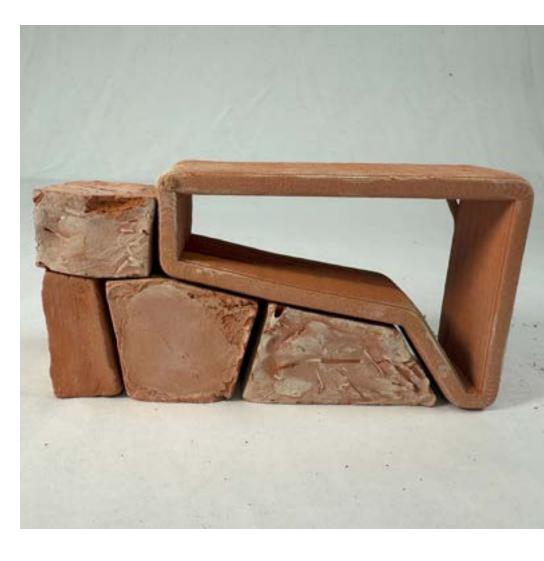
Based on my previous research regarding the ability of combustibles to increase the filtration capacity of the brick, I also tested the incorporation of fibers including reed (phragmites), oat hulls, and flaxseed.
