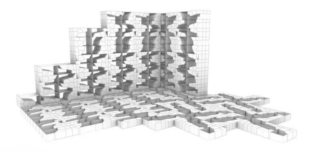
**This page: Installation Mockup**. This mockup of my installation illustrates how the module works as part of a wall, seat, path, and patio, while also working as a breeze block, waste management strategy, and water filtration system.
