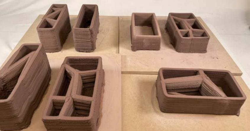
This page: 3D Ceramic Prints of Voronoi Bricks In these initial tests, I printed both 2.25" x 8" bricks and 4" x 8" bricks, using different numbers of points. This was an opportunity to consider which combination would give me the most compressive strength.
