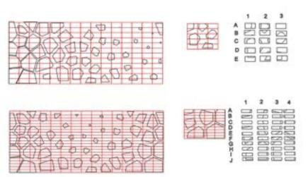
**This page: Voronoi Wall** Here, I used the voronoi in combination with the point-attract command and expirimented with breaking the result apart into different potential courses of brick. I eventually settled on a set of 12 to 3D print and test.
