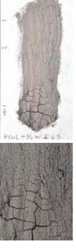
4 soil + 0 sand + 1/2 waterCRACKS > THICKNESS 2MM
