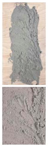
2 soil + 1 sand + 1 waterCRACKS > THICKNESS 4MM
