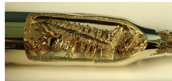
Fig. 39 Detail shot of Cesium, the main component of atomic clocks. Source: Popular Mechanics
