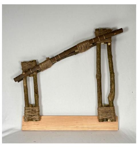
In the full-scale prototyping process, a wooden base is built to provide the foundation for the wooden sticks, which mimics the relationship between the soil and the wooden sticks. During the building of the wooden structure, the architect Anna Heringer's work METI Handmade School is referenced for the structural details, and further adjustment is applied to provide more space for the straw clay input.
