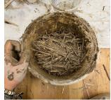
The 1:1, 1:3, and 1:6 earth-tofiber ratios are chosen to use as the input of the three small mock-up wattle frames, these three mock-ups are built to test the permeability of the frames for water management in different site situations.
