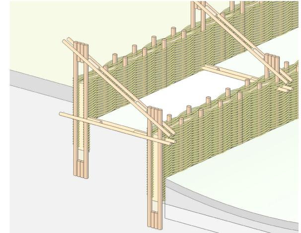
the frame, straw clay as filling, and the wooden structure as the skeleton, making the walls a self-supporting system.
