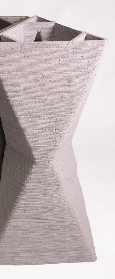
Figure 30. The initial model. However, during printing, there were inconsistencies on the upper part, resulting in the texture depicted in the image. It is fired and made of Porcelain Moist Clay and brick dust.
