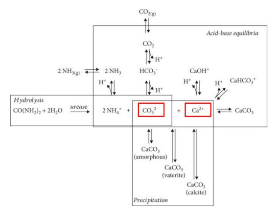
Figure 12. Chemical principles of MICP
