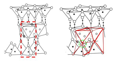
Figure 24. Left: Three-dimensional assembly of tetrahedral and octahedral sheets and formation of the 1:1 layer and the 2:1 layer. Large white circles are oxygens, large grey circles are hydroxyls, small white circles are octahedral ions and small black circles are tetrahedral ions. The image is from G.E. Christidis (2011). Right: Author's sketch
