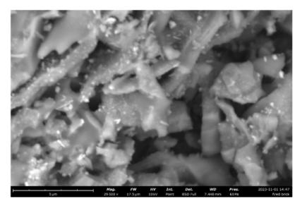
Figure 4. Structure diagram of clay (top row) and clay brick (bottom row) under SEM
