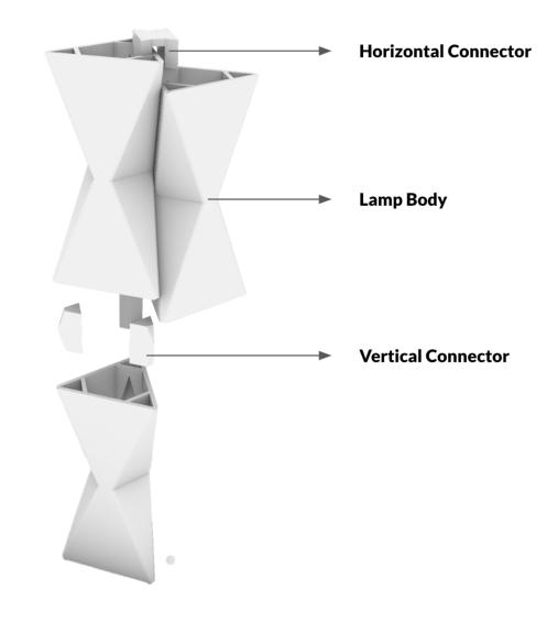
Figure 25. The connection of the modular lamp
