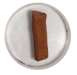
Figure 43. Brick+Casein recipe is extruded from the 3D printer.
