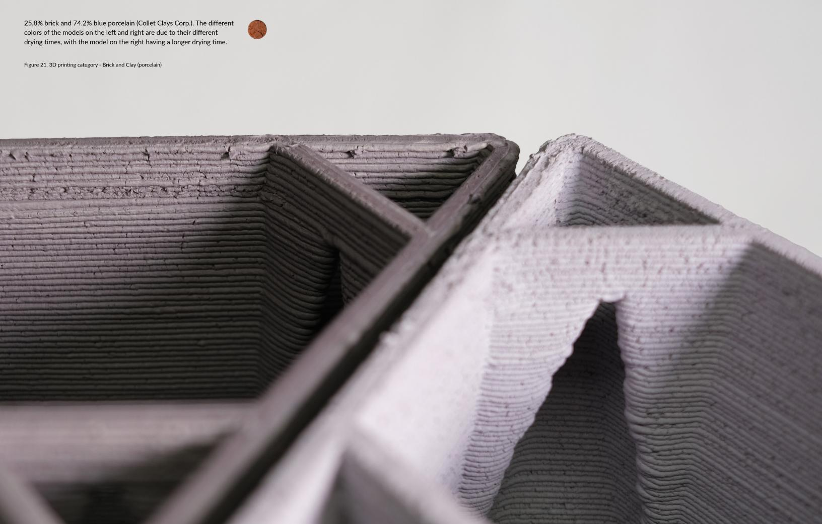
In this experiment, I added 20% clay to increase the plasticity of the mixture.
