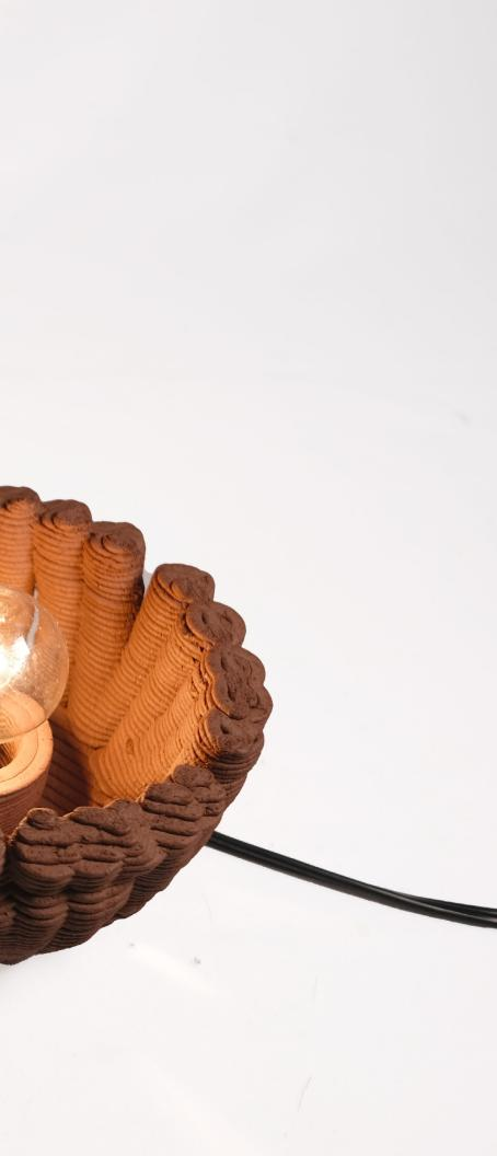
100% brick. Its characteristics are completely different from clay. It lacks plasticity and is not suitable to print for the complex modeling of 3D models.
